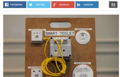
he Restroom Visitilizer System (above) tracks how heavily toilets are used, and has a sensor to measure the odour levels of things like ammonia and hydrogen sulphide. The information is then sent to a portal that can be accessed through laptops and smartphones. - The Straits Times/Asia News Network
